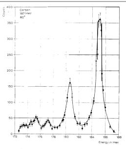
Fig. 4. This figure shows the elastic-scattering peak from carbon at an abscissa near an abscissa near the scattering peaks from the excited states of "C. The peak MeV is associated with the 4.43-MeV level."
