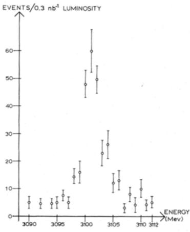
FIG. 1. Result from the Gamma-Gamma Group, total of 446 events. The number of events per 0.3 nb<sup>-1</sup> luminosity is plotted versus the total c.m. energy of the machine.
