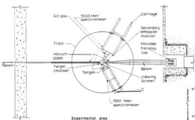
Importance of the high-density hydrogen target for proton form factor studies: pressures up to 50 atm and very thin and resistent windows
