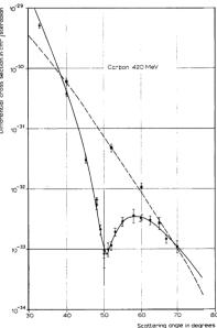
Fig. 5. This figure shows the elastic and inelastic curves corresponding to the scattering of 420-MeV electrons by "C. The *solid circles*, representing experimental points, show the elastic-scattering behavior while the *solid squares* show the inelastic-scattering curve for the 4.43-MeV level in carbon. The *solid line* through the elastic data shows the type of fit that can be calculated by phase-shift theory for the model of carbon shown in Fig. 8.
