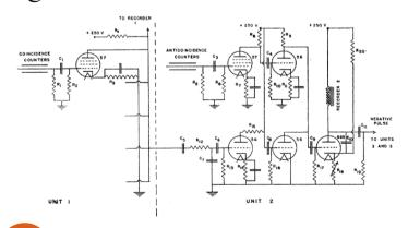
F1G. 2. Fivefold coincidence circuit (unit 1) and anticoincidence circuit (unit 2). Only one of the five Rossi tubes is shown.  $R_1 = R_6 = 10^8$ ;  $R_2 = R_6 = R_8 = 500,000$ ;  $R_4 = 500$ ;  $R_9 = 7500$ ;  $R_{10} = R_{11} = R_{16} = 2$  Meg;  $R_{11} = R_{19} = 50,000$ ;  $R_{12} = 200$ ,  $R_{11} = R_{19} = 50,000$ ;  $R_{15} = 15$ ,  $R_{10} = 10$ ,  $R_{10} =$
