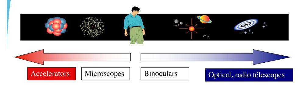
Particle physics looks at matter in its smallest dimensions and accelerators are very fine microscope or, better, *atto-scope!*  $\lambda = h/p$ : @LHC: T = 1 TeV  $\Rightarrow \lambda \cong 10^{-18}$  m = 1 a*m* (actually 30 z*m*)
