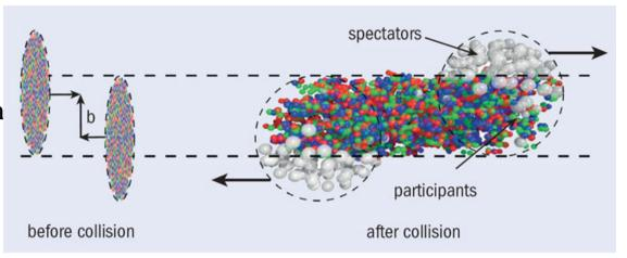
How can we experimentally measure the centrality of each event? In a heavy ion collision many particles are produced, mostly in the forward region.
