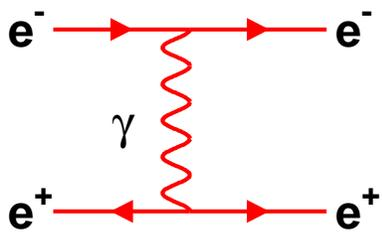
The t-channel contribution to  $e^+e^- \rightarrow e^+e^-$  dominates at small angles. Detectors typically 25 to 60 mrad from beam.
