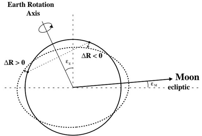
Length of orbit fixed by RF system, but magnets move with ground. Beam no longer goes through centre of quadrupoles. Sensitive to 1mm change in 27 km, typical 10 MeV peak-to-peak.
