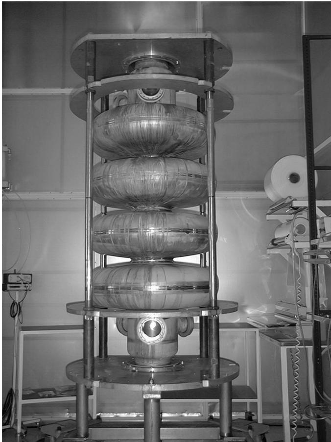
Figure 7: The  $\beta = 0.7$ , 4-cell prototype for the SPL at CERN.
