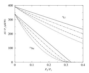
FIG. 3. Confining energy  $\Delta U$  per unit of infrared laser power for the fermionic and bosonic species as a function of the beam power ratio between the blue- and red-detuned lasers. For each species we show from top to bottom the curves obtained with the blue-detuned beams rotated with respect to the red-ones by  $\theta = 0, \pi/16, \pi/8$ , and  $\pi/4$ , respectively.
