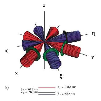
FIG. 1 (color). Combined optical dipole trap for two-species mixtures. (a) Schematic of the geometry of the two pairs of redand blue-detuned laser beams propagating along the orthogonal axes x-y and  $\xi$ - $\eta$ , depicted for the case  $\theta = \pi/4$ . (b) Relevant atomic wavelengths for the  $D_2$  lines in the case of a  $^6$ Li- $^{23}$ Na mixture and laser wavelengths for the optical trapping.
