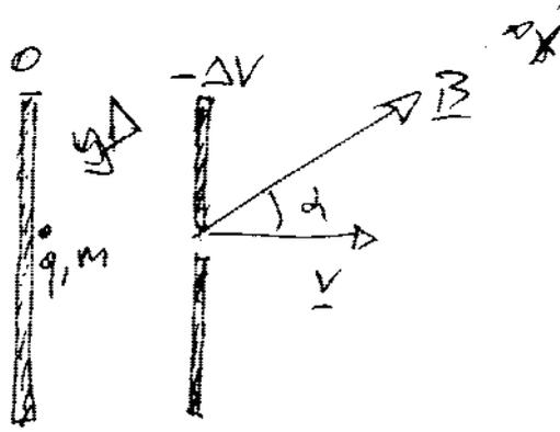
$$q\Delta V = \frac{1}{2}mv^2 \quad v = \sqrt{\frac{2q\Delta V}{m}}$$
