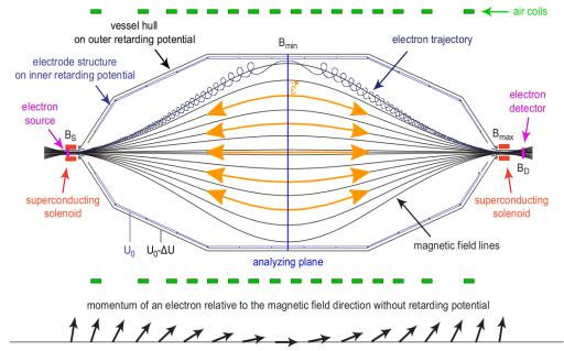
Magnetic guiding and collimation of  $e^{-}$  $\succ$  Transform  $E_{\perp}$  to  $E_{\parallel}$
