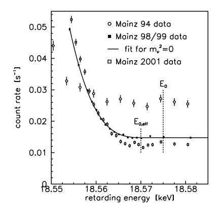
Fig. 20. Averaged count rate of the 98/99 data (filled squares) with fit for  $m^2(\nu_e) = 0$  (line) and the 2001 data (open squares) in comparison with previous Mainz data from phase I (open circles) plotted as function of the retarding potential near the endpoint  $E_0$ .
