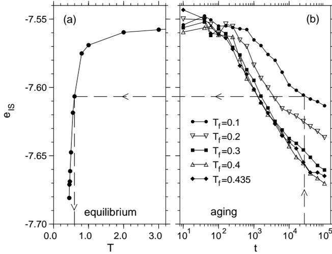
Fig. 1 –  $e_{IS}$ , the potential energy of the inherent structure in equilibrium as a function of temperature (panel a) and as a function of time during the aging process (panel b). The dashed line is used to define the effective temperature  $T_e(t)$  in the non-equilibrium case.
