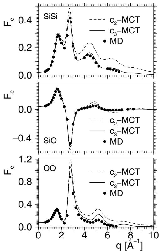
FIG. 2. The same quantities as in Fig. 1, but for silica. The MD data are from Ref. [11].
