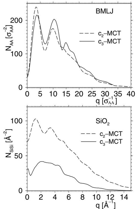
FIG. 3. Wave-vector dependence of  $N_{AA}(q, \infty)$  and  $N_{\text{SiSi}}(q, \infty)$  (upper and lower panels, respectively). The labeling of the curves is as in Fig. 1.
