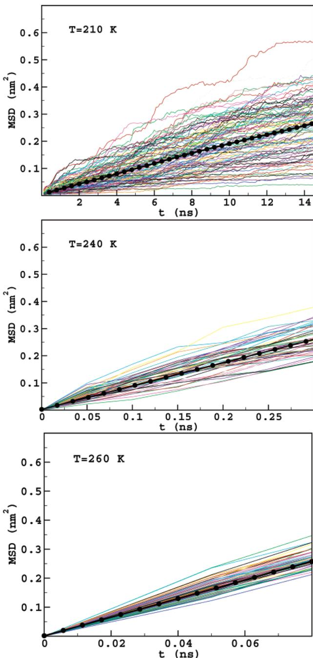
**Figure 6.** Individual mean square displacement for 100 independent realizations at three different temperatures. Filled symbols indicate the MSD averaged over the different realizations. Note that no average over starting time has been performed.
