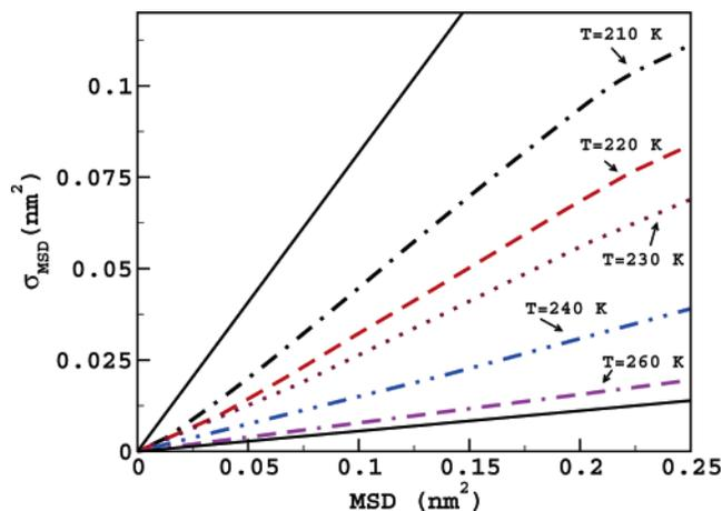
**Figure 7.** Variance  $\sigma_{\text{MSD}}$  of the MSD as a function of the average MSD for  $\rho = 0.95 \text{ g/cm}^3$ , for different  $T$ . The two full lines indicate the two extreme limits provided by eqs 11–12. Note that in water the nearest neighbor distance is 0.28 nm, corresponding to a square displacement of  $\approx 0.09 \text{ nm}^2$ .
