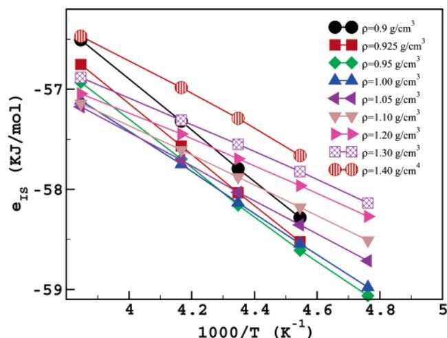
Figure 1. Temperature dependence of the average  $\langle e_{IS} \rangle(T)$  for all investigated densities.
