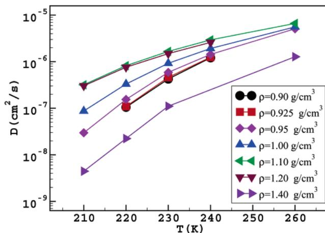
Figure 9. Average diffusion coefficient  $D$  as a function of  $T$  for several studied densities.
