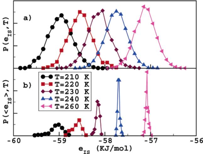
**Figure 3.** (a) Probability distribution of the  $e_{IS}$  (per molecule) at density  $d = 0.95 \text{ g/cm}^3$ , for different  $T$  values. (b) Probability distribution of  $\langle e_{IS} \rangle$ , where each average is calculated over one distinct trajectory. Units are arbitrary. Each  $P(e_{IS}, T)$  is calculated using 5000 points, because from each of the 100 independent trajectories we evaluated 50 different inherent structures, minimizing at intervals equally spaced in time.
