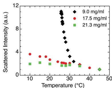
Fig. 2 Total scattered intensity as a function of  $T$  for DNA NS samples at three distinct concentrations:  $c_1 = 17.5$  mg ml $^{-1}$  (red dots),  $c_2 = 21.3$  mg ml $^{-1}$  (green squares), and  $c^* = 9.0$  mg ml $^{-1}$  (black diamonds). Data at the critical concentration  $c^*$  are from ref. 23.
