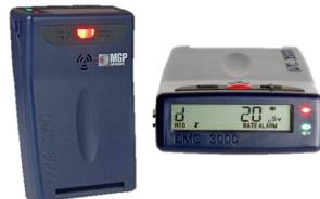
CERN Operational Dosimeter: DMC 3000 from Mirion
