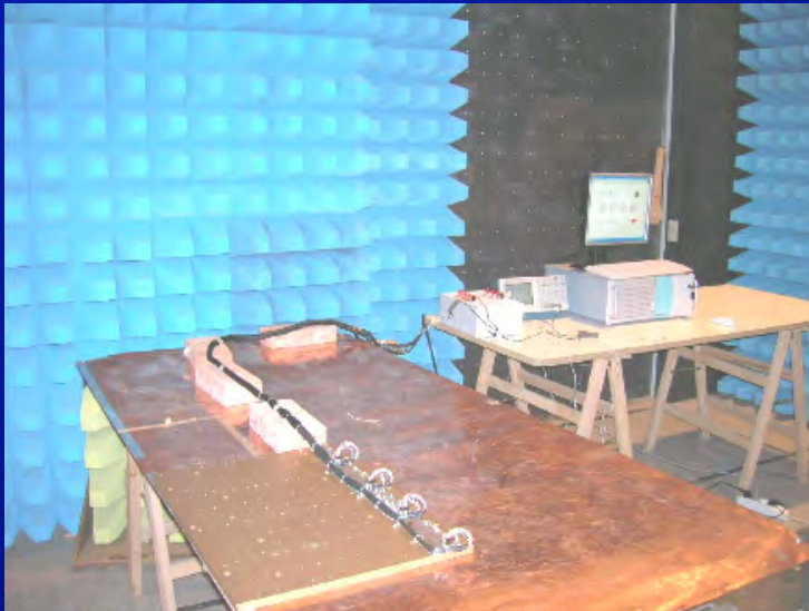
Fig. 3: Conducted Emissions, DC Power Leads, Switching Spikes (CE07).
