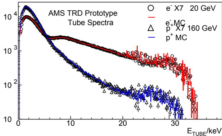
Figure 1. Energy Deposit Distributions for  $p^+$  and  $e^-$ .
