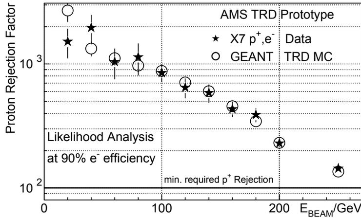
Figure 2. Proton Rejection vs. Energy.
