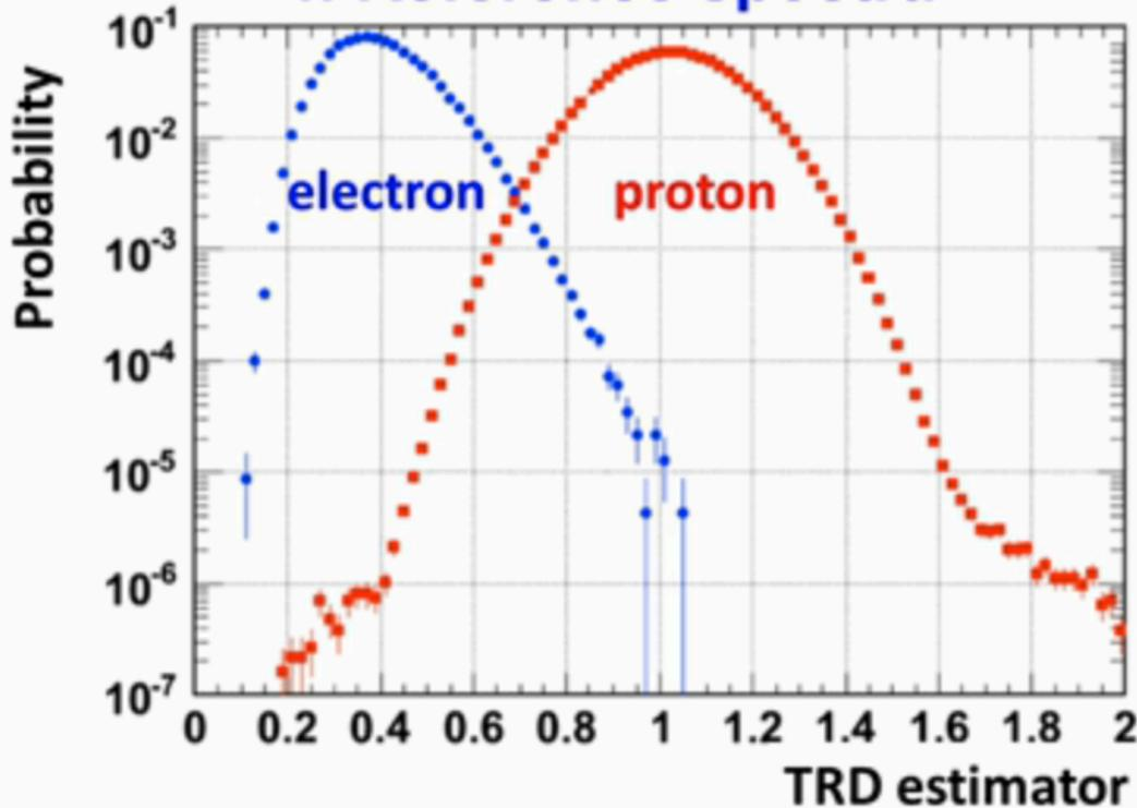
Definition of the reference spectra is based on pure samples of electrons and protons of finite statistics.
