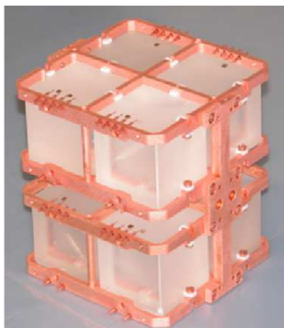
Fig. 1. (Colour on-line) A small bolometric array (named RAD) used for test purposes: an eight-crystal array mounted inside its Cu holder. The \text{TeO}_2 crystals have a mass of 790 g each and the detector is completed by a Cu full coverage here removed.
