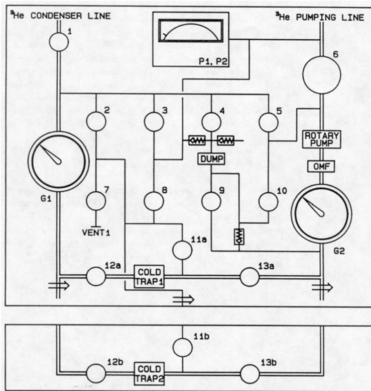
Fig. 11: Auxiliary system schematic
