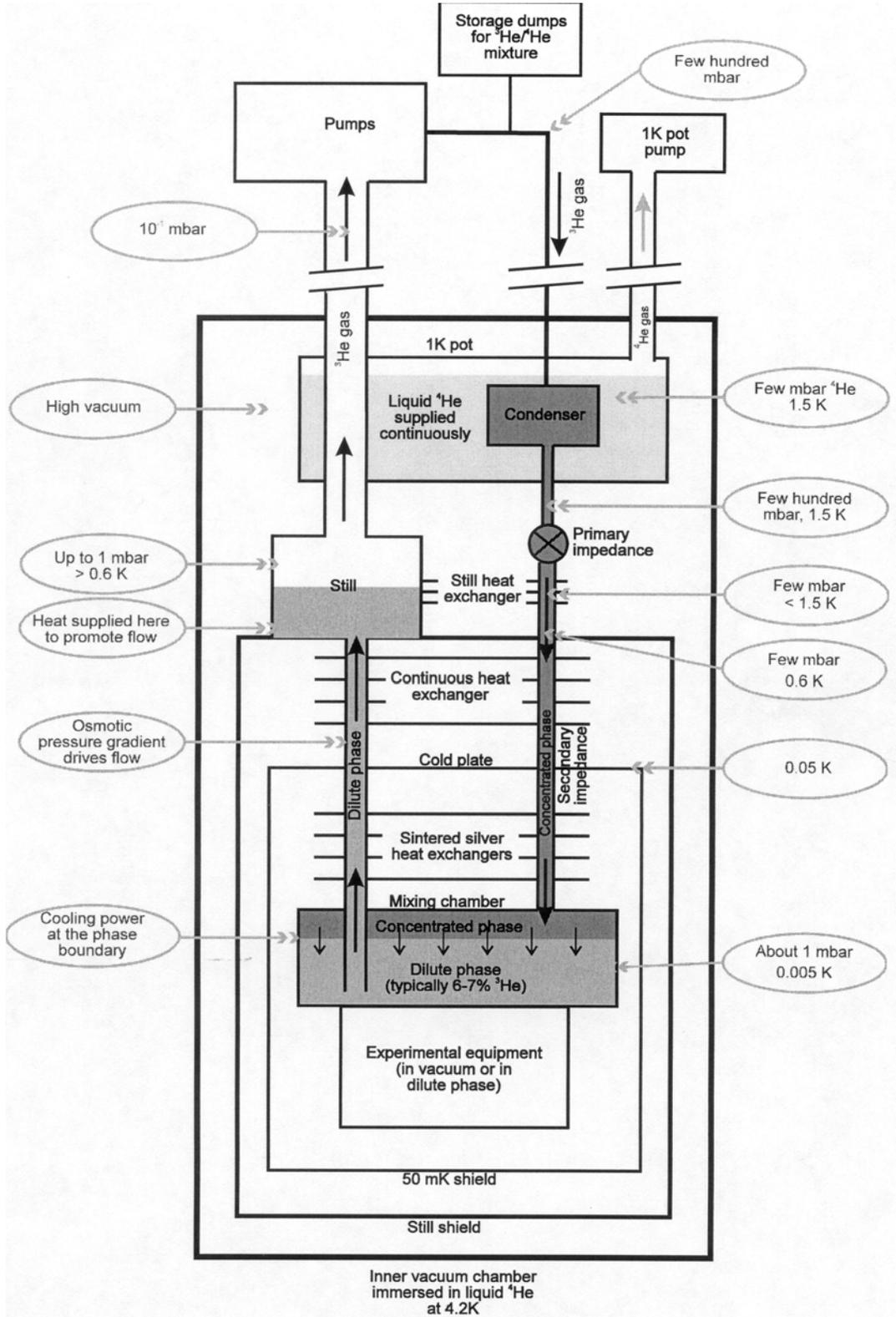
Fig. 10: Circulation system schematic
