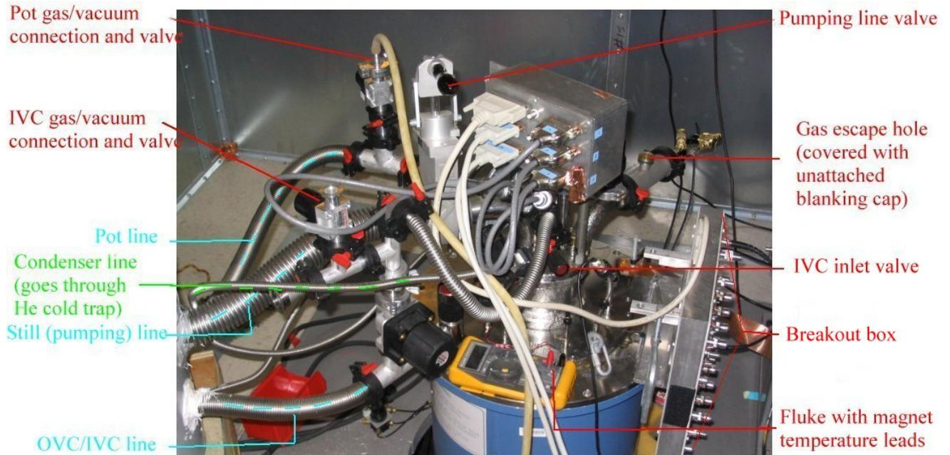
Fig. 2: Back side of dilution refrigerator
