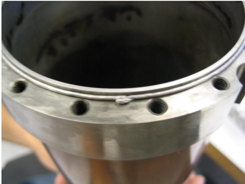
Fig. 7: Insert without inner radiation shield
