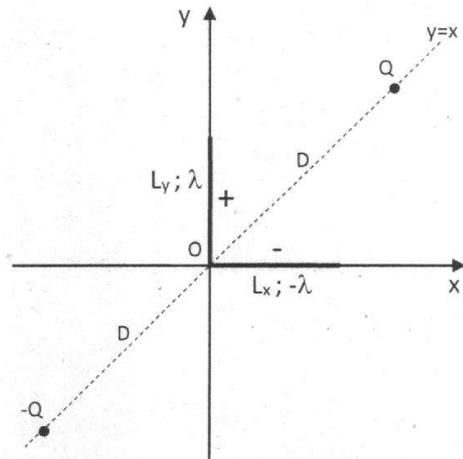
Dati:  $L = 10 \text{ cm}$  ;  $\lambda = 1 \mu\text{C/m}$  ;  $Q = 1 \mu\text{C}$  ;  $D = 3 \text{ m}$ .
