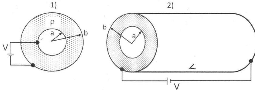
$$I_1 = \frac{V_0}{R_1} ; \quad I_2 = \frac{V_0}{R_2} \quad R_2 = \frac{\rho L}{S} = \frac{\rho L}{\pi(b^2 - a^2)} \quad [2]$$
