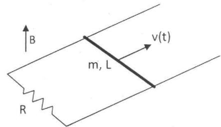
$$m = 10g; \quad L = 10\text{ cm}; \quad B = 0,5\text{ T}; \quad R = 4\Omega$$
