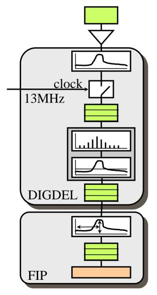
Detector Amplifier Shaper Sampling 4 raw data banks. Digital filter Zero suppression **Buffer** Feature extraction **Buffer** Format & Readout
