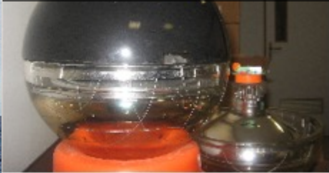
The OM: 10" Hamamatsu R7081, Front End Module, Time Calibration, LED beacons
