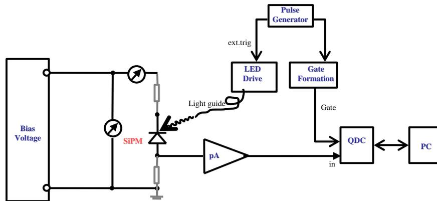
Figure 1. The static polarization circuit (on the left part), the pulsed light injection circuit (on the middle) and the readout via an integrating ADC circuit (on the right) are shown.
