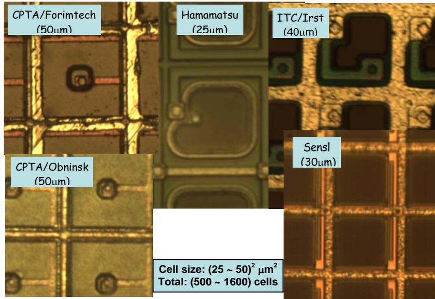
Figure 2. A mosaic of five photos taken by a microscope of the five tested SiPM is shown. To be noted that the shown photos are not in scale. The matrix structure is evident. The packages are TO5 for SenL and TO8 for the others.
