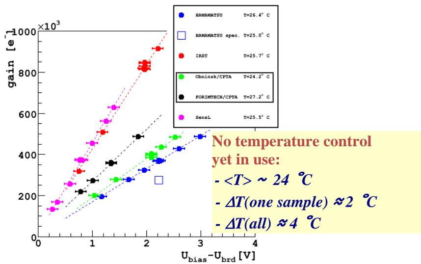
Figure 4. Gain as a function of the over voltage ( $V_{\text{bias}} - V_{\text{breakdown}}$ ) for the tested SiPM is reported.
