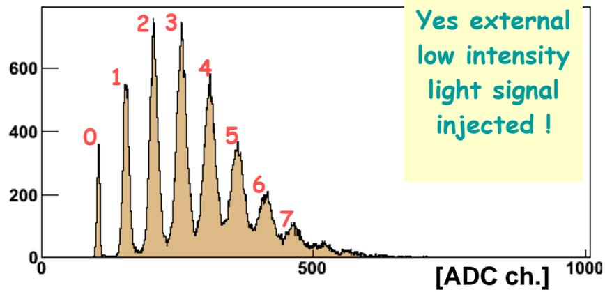
Figure 3. Typical raw pulse height spectrum (in terms of ADC counts) obtained from one SiPM pulsed by a low intensity LED light. On the reported spectrum the multi peak structure refers to the various numbers of fired cells in a particular triggered light pulse impinging the matrix.
