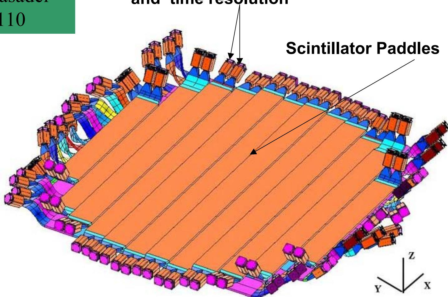
**Scintillator Paddles With Phototubes at Both Ends**
