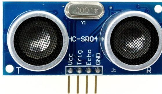
**Figure otto.3** : The HC-SR04 sensor is an ultrasonic model composed by a speaker and a microphone. It can be used to measure distances.
