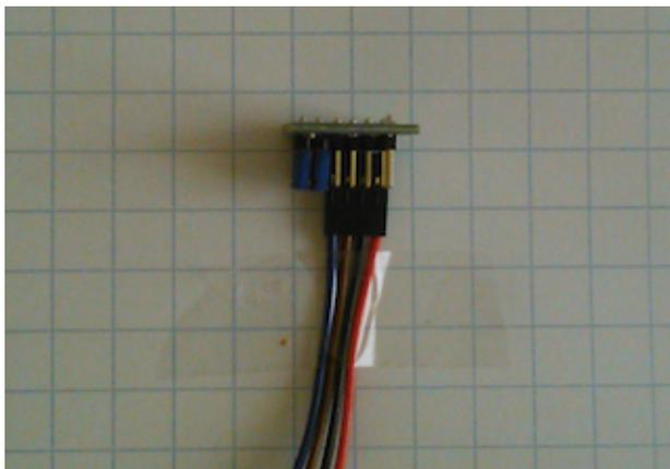
**Figure otto.8** The digital compass can be firmly placed on a piece of paper just using a strip of scotch.
