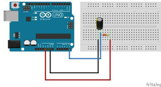
**Figure otto.1** An RC circuit connected to **Arduino**.
