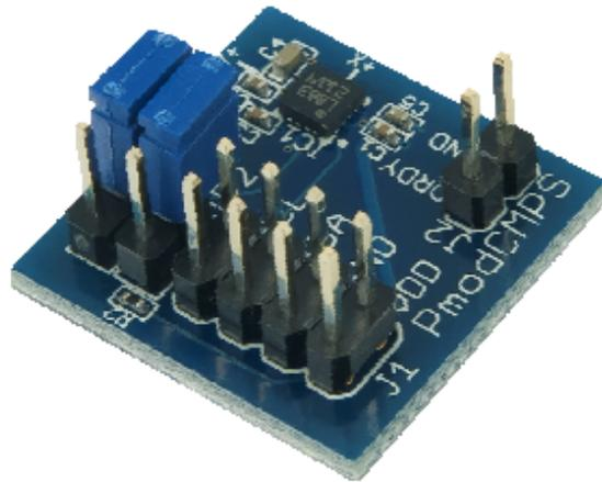
**Figure otto.6** The PmodCMPS module: a digital compass to measure magnetic fields.
