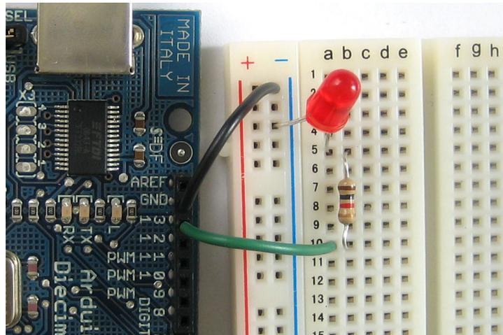
**Figure sette.3** An Arduino board with a red LED connected to pin 13 through a 100 Ω resistor.
