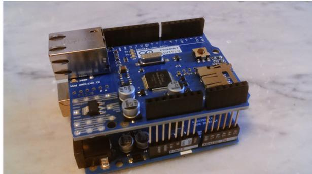
Figure sei.2 An Arduino board with an Ethernet shield mounted on it.
