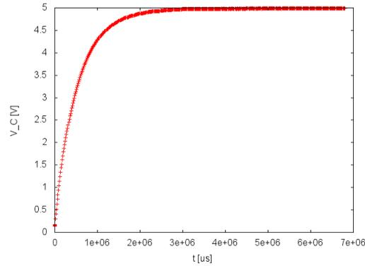
**Figure otto.2** The voltage across the capacitor of an  $RC$  circuit versus time.
