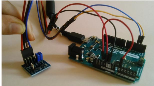
Figure otto.7 Connecting a digital compass to an Arduino Leonardo board.
