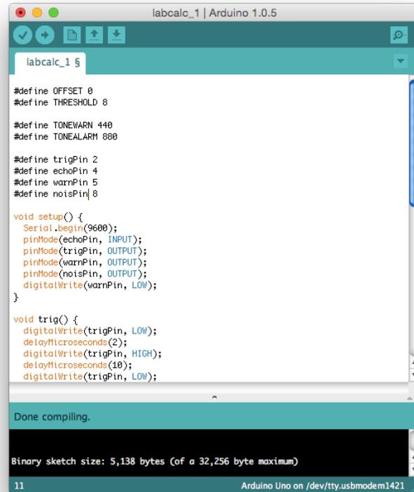
**Figure due.2** The Arduino IDE appears as a window in which you can type the text of the program, called **sketch**.
