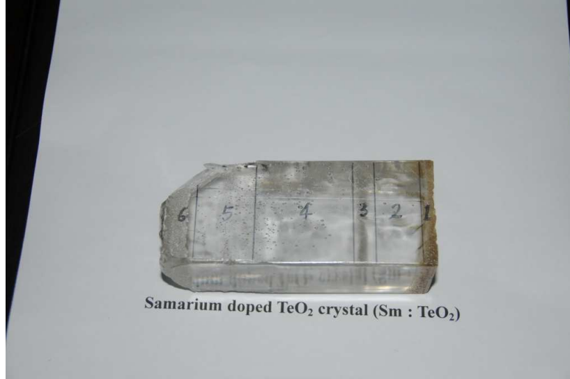
Figure 1. Sm doped \text{TeO}_2 crystal as grown. Different samples were cut for analysis. The cloudy (no. 3) region is due to a thermal instability during the growth process.
