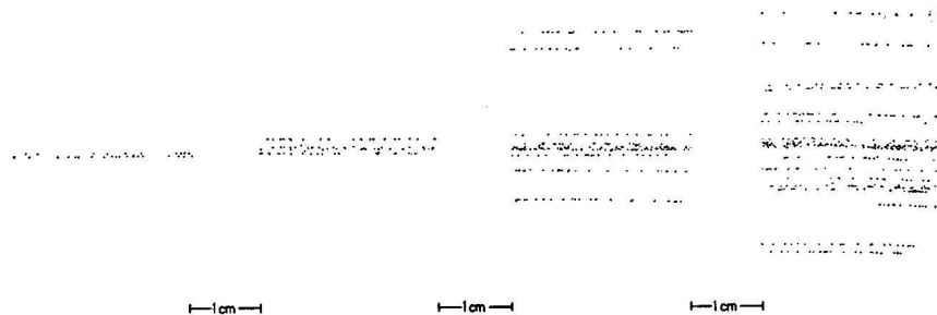
FIG. 1. Narrow shower of pure photons. Sections at arbitrary intervals to show development of shower. Note pair starting in last section.
