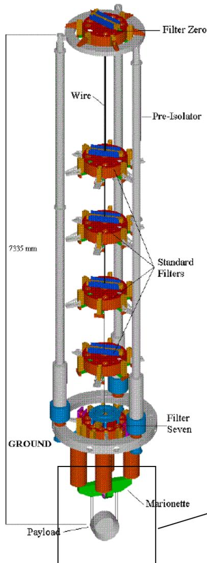
**Superattenuator:** A chain of pendula in all DOF, filtering the seismic noise in all directions.
