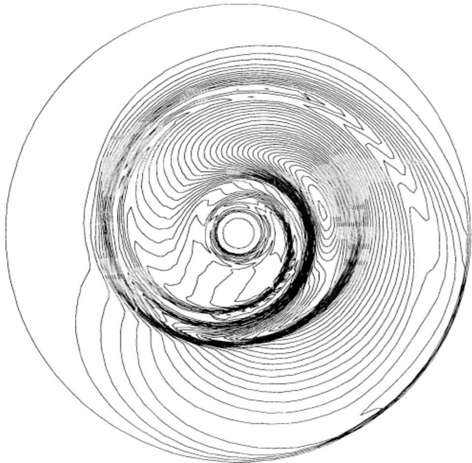
**Manifestation of the PPI:** counter-rotating epicyclic vortices, or "**planets**", with  $m$  planets emerging from the growth of a mode of order  $m$ .
