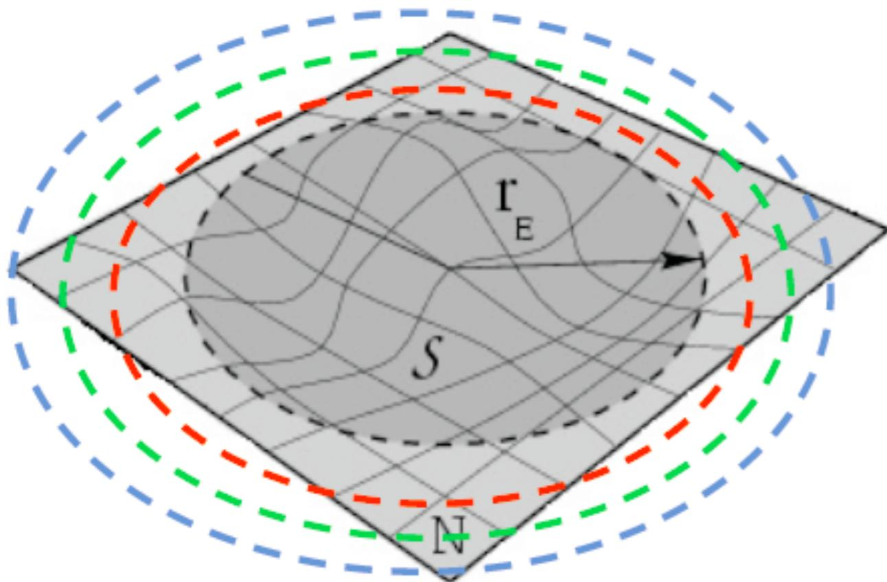
In both approaches **observers** are located at various positions from the source (nested spheres), where **Weyl scalars** are computed or where the metric is decomposed in tensor spherical harmonics to compute **gauge invariant perturbations** of a Schwarzschild black hole.
