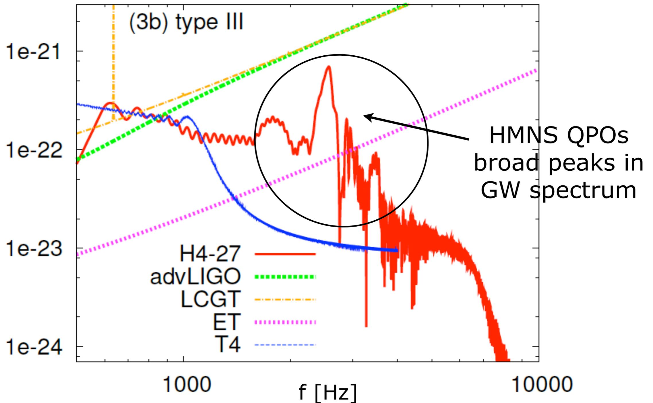
2-4 kHz peaks in spectrum detectable by 3rd generation detectors (ET) or advLIGO if source closer (20 Mpc)
