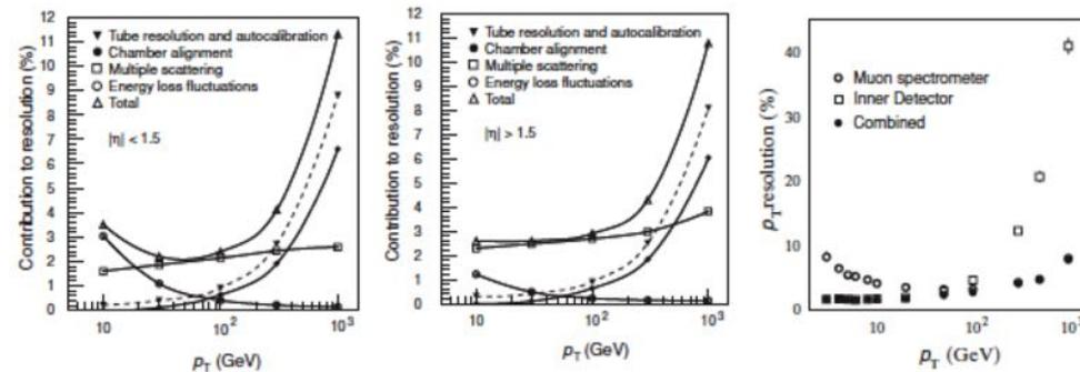
Figure 24 Expected performance of the ATLAS muon measurement. Contributions to the momentum resolution in the muon spectrometer averaged over  $|\eta| < 1.5$  (left) and  $1.5 < |\eta| < 2.7$  (center). (Right) Muon momentum resolution expected from muon spectrometer, Inner Detector, and their combination together as a function of muon transverse momentum.
