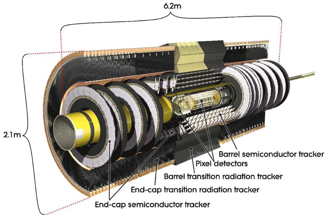
**Figure 1.2:** Cut-away view of the ATLAS inner detector.
