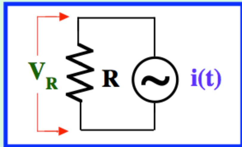
$$i(t) = I_0 \sin(\omega t) \rightarrow V(t) = V_0 \sin(\omega t + \phi')$$
