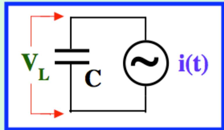
$$i(t) = I_0 \sin(\omega t) \rightarrow V(t) = V_0 \sin(\omega t + \phi')$$
