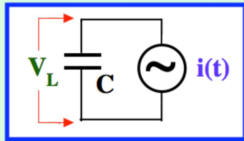
$$Q(t) = \int I_0 \sin \omega t \, dt = - \frac{I_0}{\omega} \cos \omega t$$
