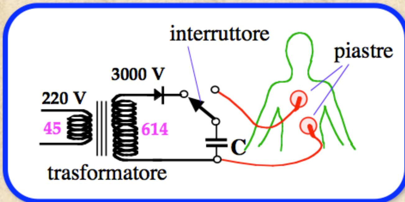
$$V_{o2} = \frac{N_1}{N_2} V_{ol} = \frac{614}{45} 220 \text{ V} = 3000 \text{ V}$$
