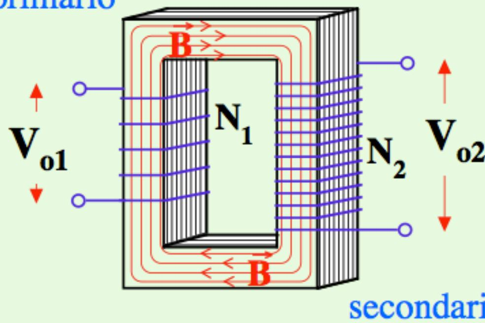
$$\frac{V_{o1}}{V_{o2}} = \frac{N_1}{N_2}$$
