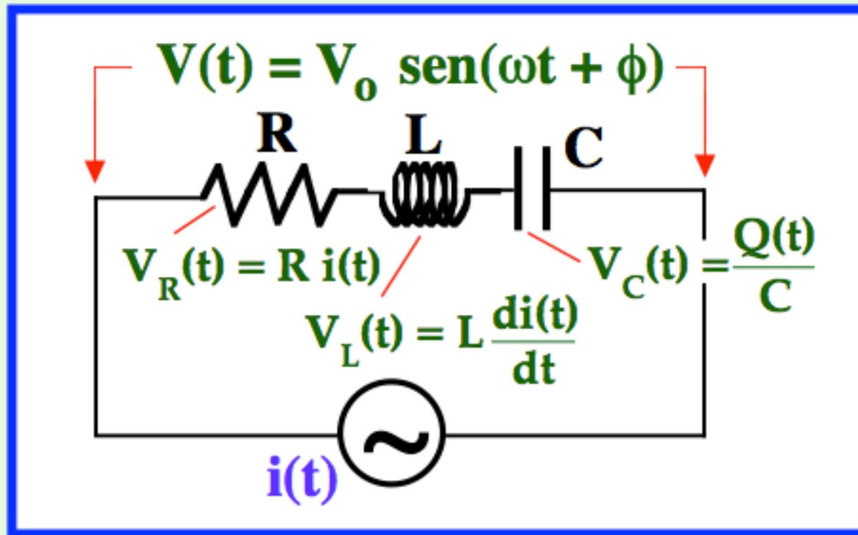
$$i(t) = I_0 \operatorname{sen}(\omega t) \rightarrow V(t) = V_0 \operatorname{sen}(\omega t + \phi)$$
