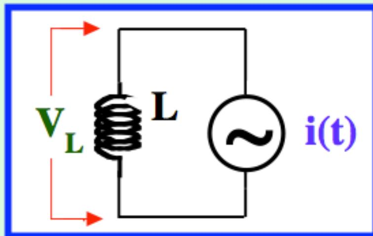
$$i(t) = I_0 \sin(\omega t) \rightarrow V(t) = V_0 \sin(\omega t + \phi')$$
