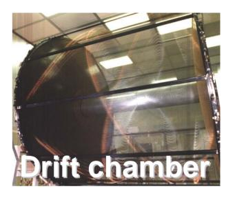
4 m diameter × 3.3 m length 90% helium, 10% isobutane 12582/52140 sense/total wires All-stereo geometry
