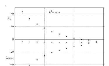
Lyapunov spectra for NS with normal viscosity (N=5 truncation) at  $R^2=2222$  (left) and  $R^2=5000$  (right), and corresponding GNS runs with constrained energy  $Q_0$ . The 2K-2 nontrivial exponents are drawn by associating each value of the abscissa  $k=1,2,\ldots,K-1$  with the k-th largest exponent  $\lambda_k$  and the k-th smallest exponent  $\lambda_k' = \lambda_{2K-k-1}$ . Symbols
