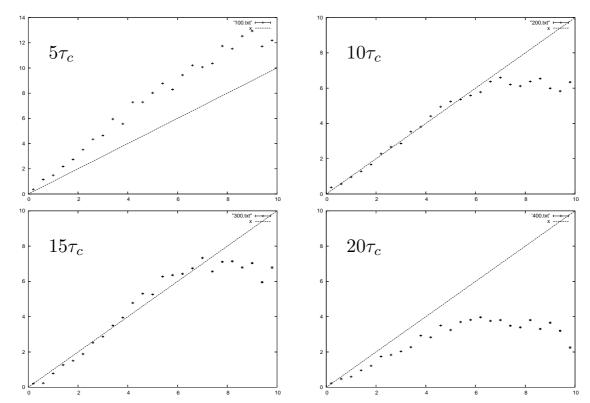
Results for  $\tau = 5, 10, 15, 20$  times  $\tau_c$  for the turbulent flow ( $\sim 20ms$ )
