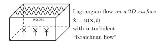
The water in a container of  $1m \times 1m \times 0.3m$  size is set into a turbulent state. generate the "lagrangian trajectories" of the surface flow, solutions of the equations
