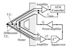
Block diagr. of feedback system from [48] (Nakabeppu-Suzuki:) a "thermometer" operating above room temperature and performing on a scale of  $10\,nm=100A^o$  (the size of one Hydrogen atom is .1nm or  $1\,A^o$ ).
