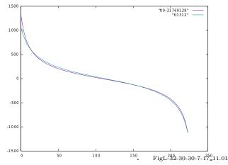
Graph of the Lyapunov spectra in a  $15 \times 15$  truncation for the NS2D with viscosity and reversible viscosity (captions ending respectively in 0 or 1) with (the 224 points) interpolated by lines, R = 2048. Preliminary
