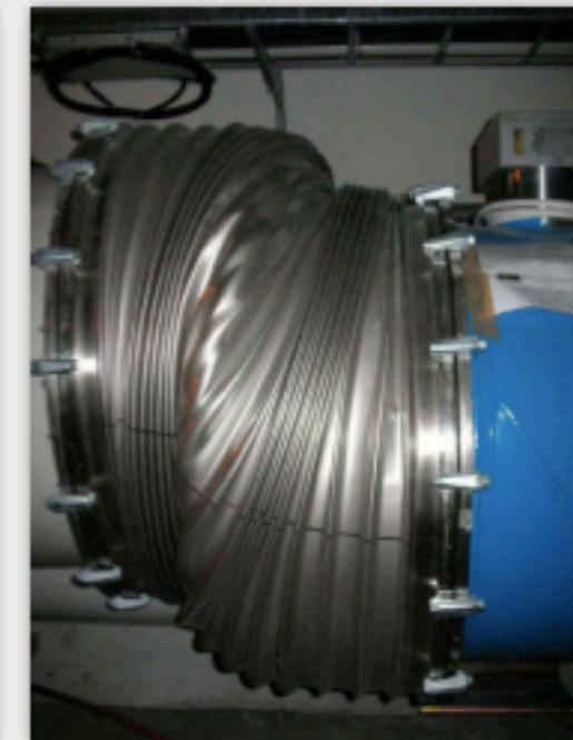
2 most severely damaged interconnects
