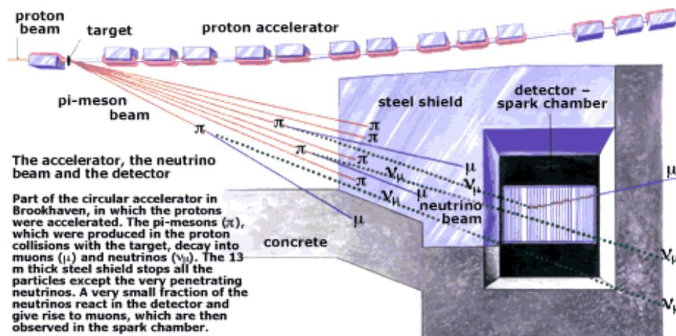
**The accelerator, the neutrino beam and the detector**
