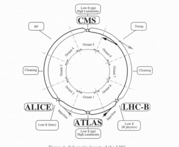
Figure 1: Schematic layout of the LHC
