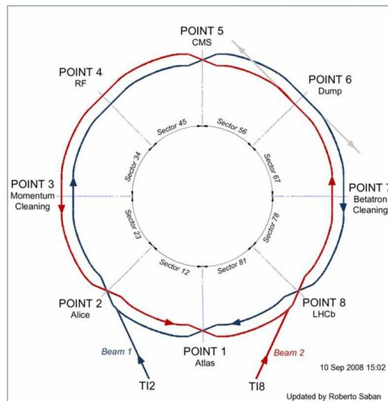
Figure 4 – LHC beam layout.
