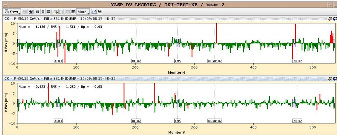
Figure 11 – Corrected closed orbit on B2. Energy offset of  $\sim -0.9$  permil due to the capture frequency.
