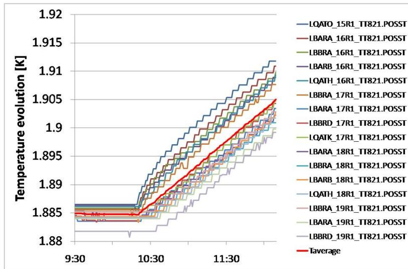
Figure 15 – Experimental validation: temperature evolution.
