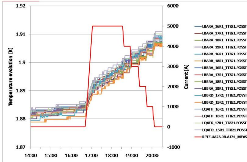
Figure 16 – Powering example: 15R1 powering @ 5000A.
