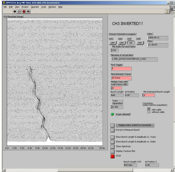
Figure 9 – Capture with corrected injection phase but wrong frequency.
