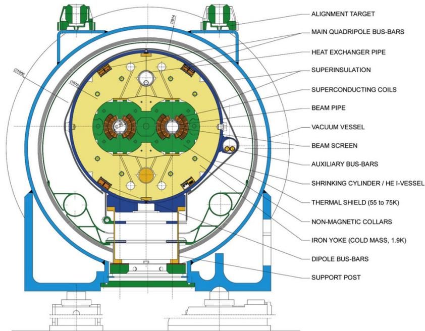
Figure 2 – LHC dipole cross-section
