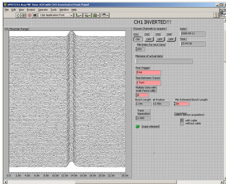
Figure 10 – Capture with optimum injection phasing, correct reference.
