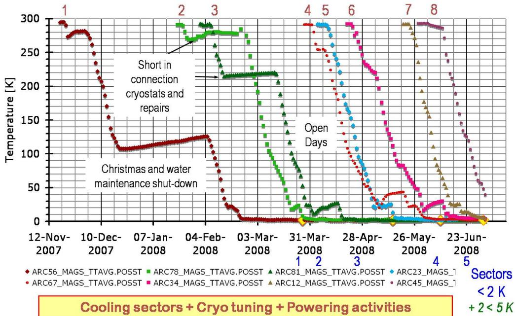
Figure 3 – Cooldown of LHC sectors.
