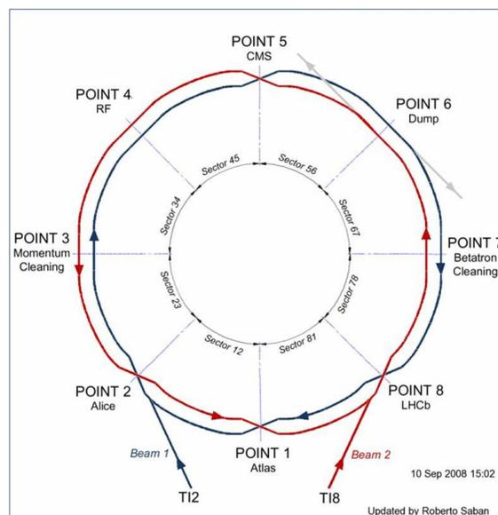
Figure 4 – LHC beam layout.
