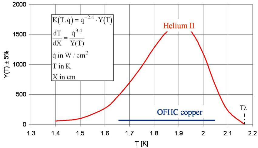
Figure 12 – Equivalent thermal conductivity of He II.
