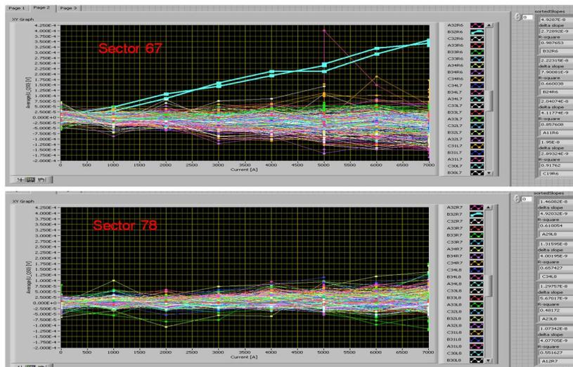
Figure 17 – Snapshots in S67 and S78 on all 154 dipoles - B32.R6 with a high (47 nΩ) joint resistance between the poles of one aperture.
