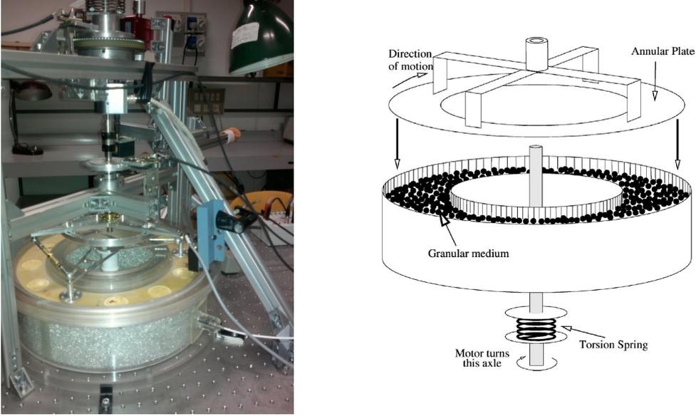
Fig. 6. – An image of the laboratory granular system and its schematic.
