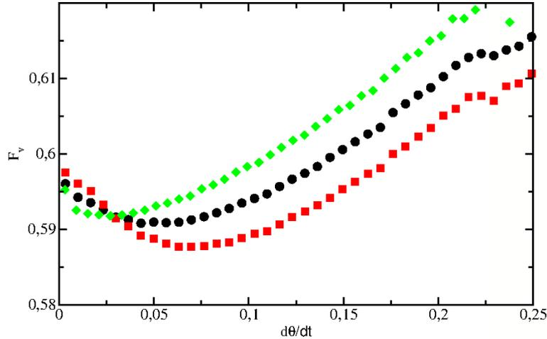
Fig. 13. – Friction torque measured in an experiment with imposed plate speed. Diamond (green on line) correspond to increasing speed and square (red on line) to decreasing speed. Bullets (black) are the average friction.
