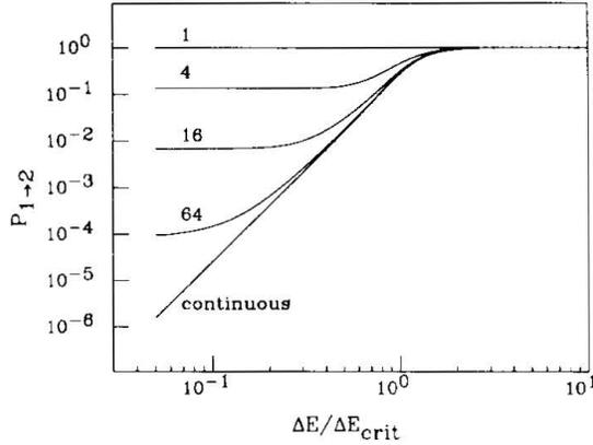
Fig. 2. Transition probability  $P_{1 \rightarrow 2}$  at the end of an on-resonance  $\pi$  pulse versus the normalized measurement error  $\Delta E / \Delta E_{\text{crit}}$  for pulsed measurements with 1, 4, 16, 64 pulses and a continuous measurement.
