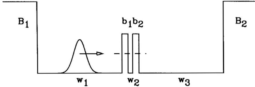
Figure 1: Energy diagram of a three-well two-barrier heterostructure. The barriers  $b_1$  and  $b_2$  separated by the well  $w_2$  produce a resonance in the currents between wells  $w_1$  and  $w_3$  at the energy indicated by the dashed line. An electron cloud is initially localized in the well  $w_1$  and moves toward the well  $w_3$  with a mean kinetic energy close to the resonance.
