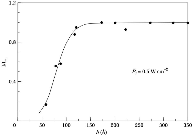
**Fig. 1.** Normalized photoluminescence ratio  $III_{\infty}$  of a near-surface well versus the surface-barrier thickness  $b$ . Dots: experimental data from Ref. [1]; solid line: best fitting in terms of the self-consistent model. Incident power density is  $P_i=0.5 \text{ W cm}^{-2}$ .
