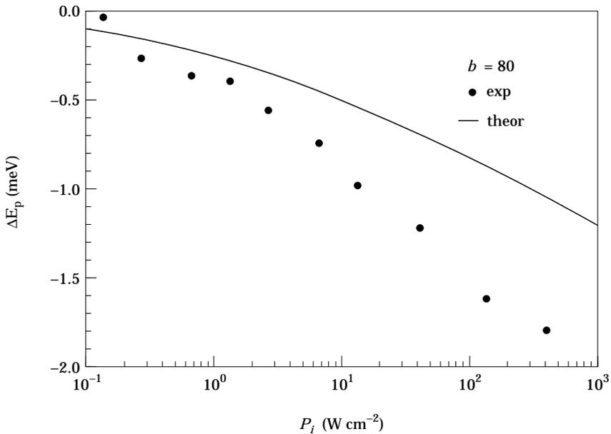
**Fig. 3.** Comparison between the Stark shift of the photoluminescence signal calculated from the model (solid line) and measured (dots) versus the incident power density  $P_i$ . The surface-barrier thickness is  $b = 80 \text{ \AA}$ .
