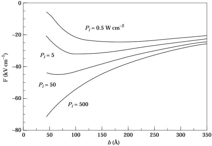
**Fig. 2.** Calculated electric field  $F$  across the surface barrier versus the surface barrier thickness  $b$  for different incident power densities  $P_i$ .
